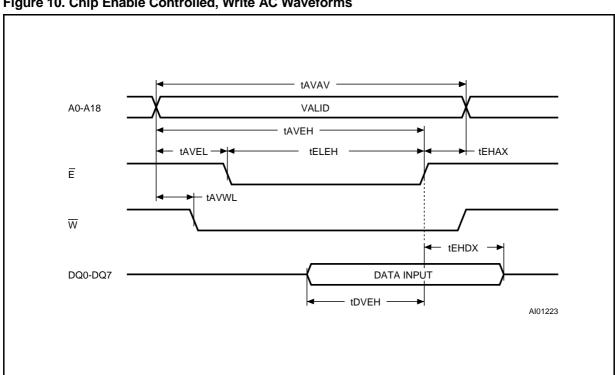
Figure 10. Chip Enable Controlled, Write AC Waveforms
