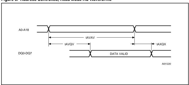
**Note:** Chip Enable  $(\overline{E})$  and Output Enable  $(\overline{G})$  = Low, Write Enable  $(\overline{W})$  = High.
