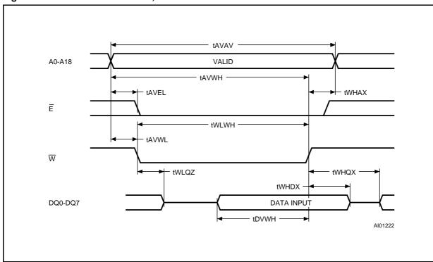
Figure 9. Write Enable Controlled, Write AC Waveforms
